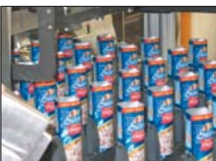
PSG ABT 6 Lane Transverse machine, filling and sealing Premade StandUp Retort/shelf stable Chicken pouches.
