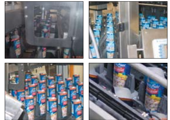
PSG ABT 6 Lane Transverse machine, filling and sealing Premade StandUp Retort/shelf stable Chicken pouches.
