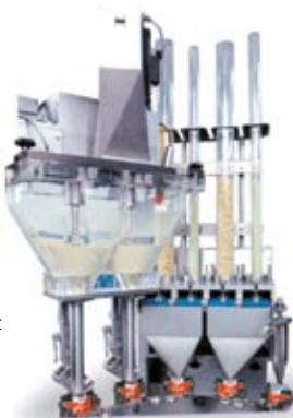
3-Component Dosage Duplex Filling
