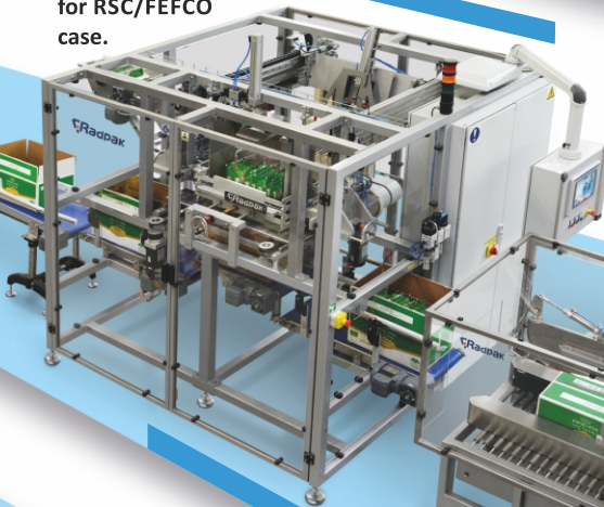
Wide range of RSC / Retail Ready Display Cases formed on Servo Case Packer.
