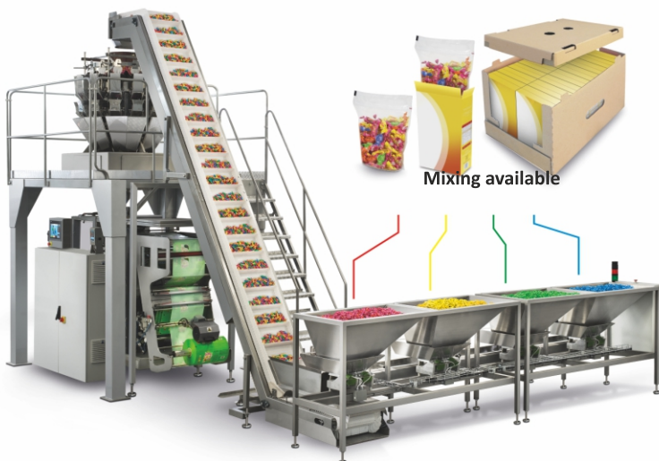
Packing line for quad bags designed to pack sweets.
