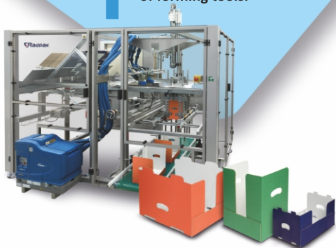
Tray former RT-01 Servo driven with quick change of forming tools.
