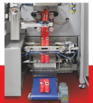
VFF&S Machine RM-32ACD Doypack with rotated horizontal jaws with zipper applicator.
